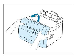
**CAUTION:** To prevent damage to the toner cartridge, do not expose it to light for more than a few minutes. Place a piece of paper over the top of the toner cartridge to shield it while it is out of the printer.
